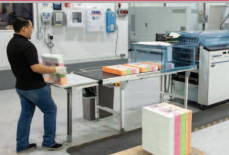
**Darwill installed a Hunkeler UW6 Unwinder on the front end of its new ProStream 1000 Press. On the back end, the DP8-II Dynamic Perforator feeds into a CS8-II Rotary Cutter and LS8 Stacker to deliver cut sheets ready for further finishing.**
