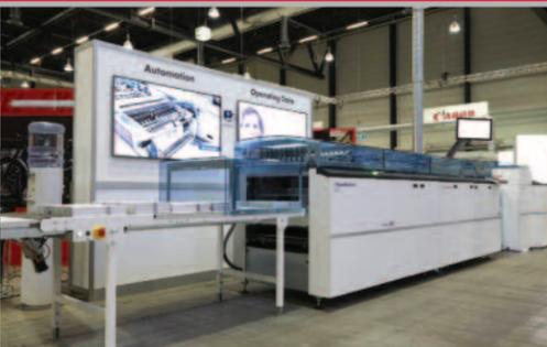
*The Hunkeler Gen8 Roll-to-Cut/Stack solution features fully automated, no-touch changeover between 1-up, 2-up, 3-up, and 4-up stacks, resulting in significant cost savings due to reduced changeover time. At the show, book blocks were being finished on the near-line Horizon BQ-480 Perfect Binder.*
