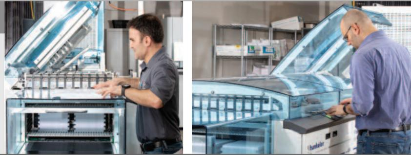
With a new press and in-line Hunkeler finishing, BIP has significantly ramped up its production. They anticipate producing about 450,000 perfect bound books in 2019. Using three or four rolls of paper per day, an equivalent of about 300,000 sheets, the Standard Horizon BQ-470 Perfect Binder with HT-80 Trimmer (far right) can handle that volume with room to spare.
